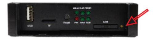
8. Insert your sim card onto the SIM cradle and reinstall the cradle.
